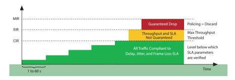
Service configuration test (ramp test) validates each service/stream
