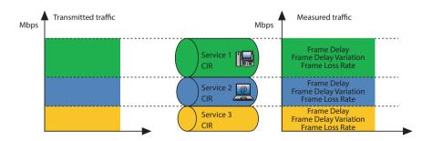
Service-performance test (multistream) tests all streams simultaneously
